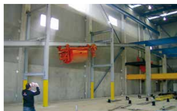
Rollover bucket 4000 l in a 10° inclination
