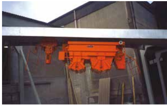
Double chamber - bucket for two concrete types
