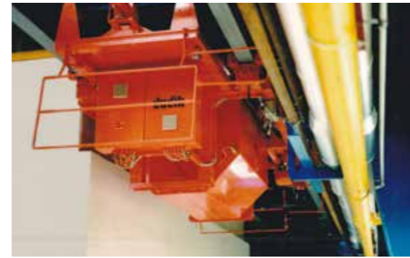
Heated bucket, up to 150° C
