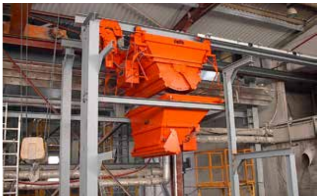
Flap bucket / Transfer silo 5000 l
