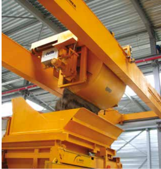
Distributor bucket in a bridge 25 m
