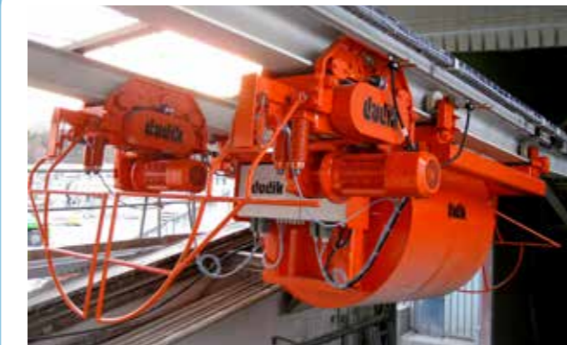
Rollover bucket 2000 l in a 20° inclination
