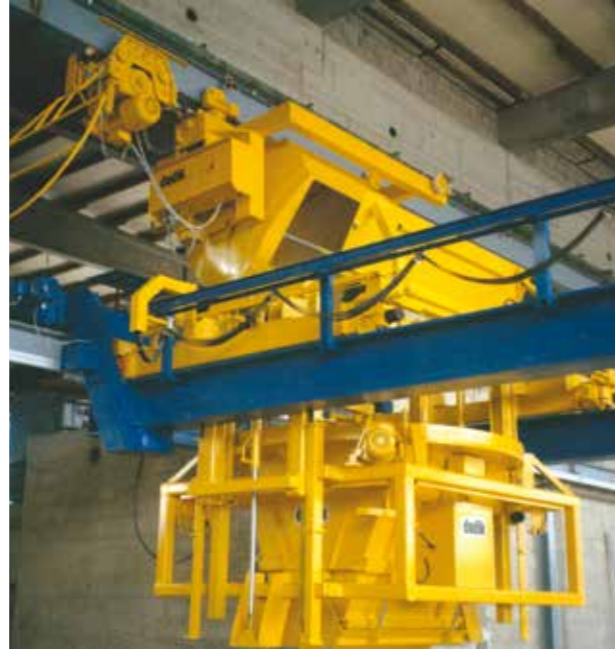
Distributor bucket 180° rotatable
