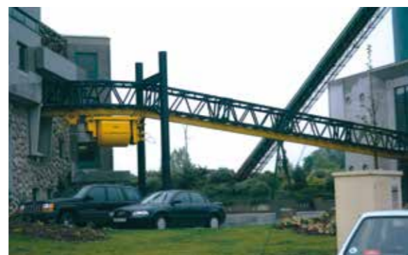
Rollover bucket 3000 l in a bridge 25 m
