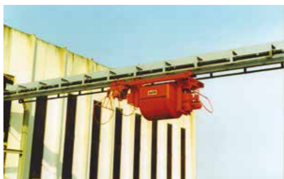
Rollover bucket 2500 l in a bridge 20 m
