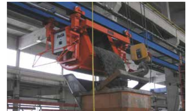
Directly discharge into crane bucket
