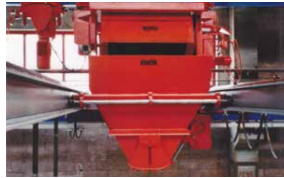
Discharge rollover bucket into a distributor
