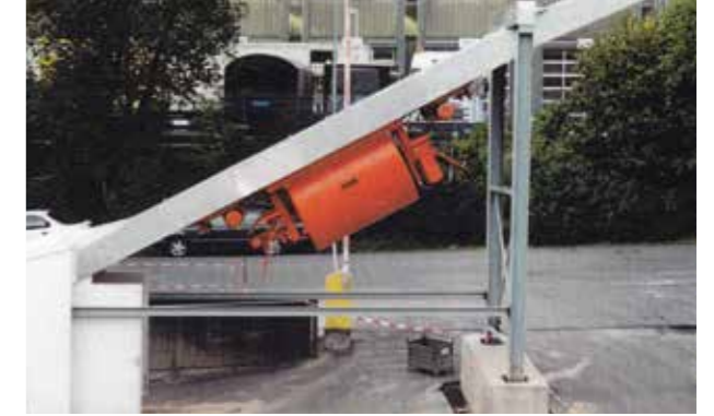
Rollover bucket 3500 l in a 30° inclination
