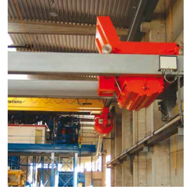
Half portal, span width 23 m
