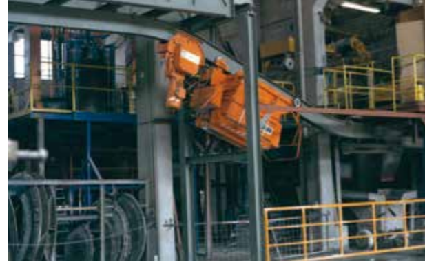
Inclination after the mixer 30°
